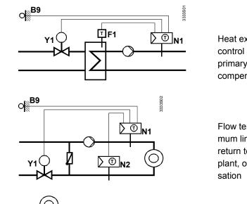
Heat exchanger control through control of the 2-port valve in the primary flow, outside temperature compensation
