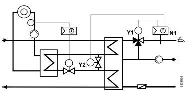
Direct DHW heating via heat exchanger, Y1 controls the mixing valve in the DHW circuit, Y2 controls the 2-port valve for DHW priority
