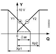
$\Delta w$ Setpoint difference Q Heating or cooling load
